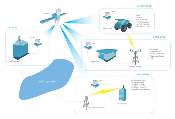
Whether secure site-to-site or high performance site-to-multi-site, a VSAT network infrastructure from Vizocom is highly scalable. It delivers a cost-effective, high performance communications platform whether for only a few sites in a single geographical region or to provide connectivity to hundreds of sites globally.
